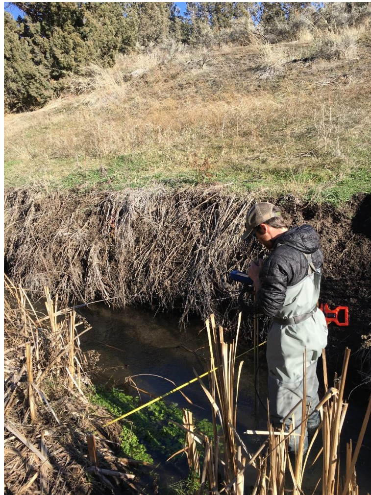
Measuring stream flow on Campbell Creek as part of the Pesticide Stewardship Partnership monitoring.
